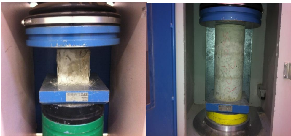
Figure 2 Compressive strength Test using Avery Denison 2500 kN machines.
