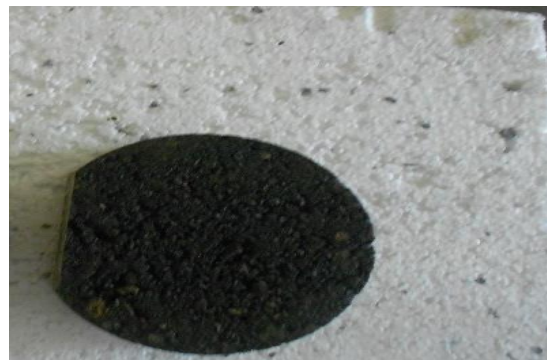
Figure 3: Specimens for HWT Test
