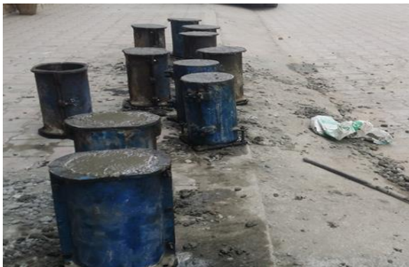
Figure 3: Concrete Cylinders Casted
