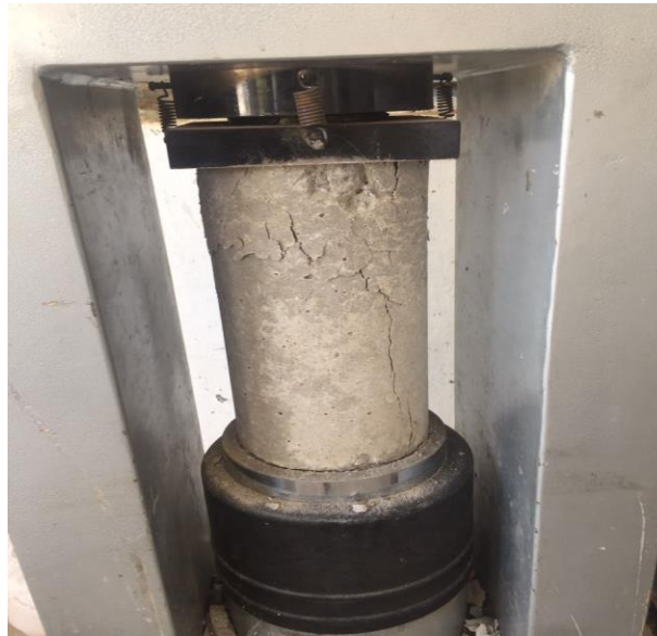
Figure 5: Compression test of cylinder
