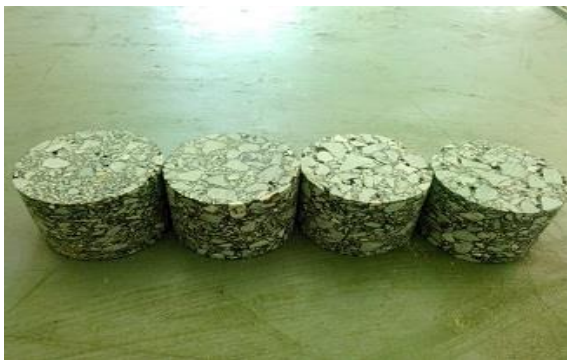
Figure 2: Specimens for IDT and MR Tests
