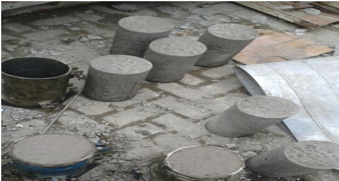
Figure 2: Casting of cylinder
