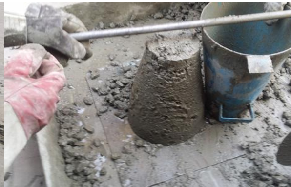
Figure 4: Measurement of Slump
