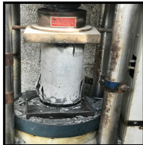
Figure:2 Crushing of Trial Specimen
