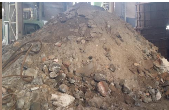
Figure 2: UFS After Demoulding
